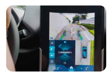
Jelly View allows drivers to gain a clear view beneath their vehicle. The view is constructed using images from sensors and cameras, enabling Jelly View to be seamlessly integrated into existing vehicles without additional hardware.
