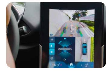
Jelly View allows drivers to gain a clear view beneath their vehicle. The view is constructed using images from sensors and cameras, enabling Jelly View to be seamlessly integrated into existing vehicles without additional hardware.
