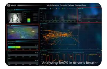
DrunkSense uses a multi-sensor approach that combines input from the DMS camera, such as tracking eye movement and blinking, with vehicle information like braking and acceleration control, to capture the complete views of drivers' behaviors. DrunkSense has 85% sensitivity in drunk driver detection, 8% higher than industry standards.
